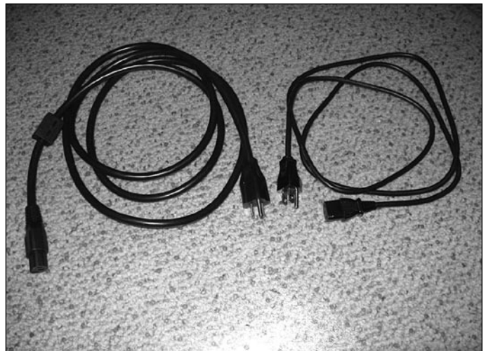
PHOTO 12: Power cords—14 gauge vs. 18 gauge stock.
