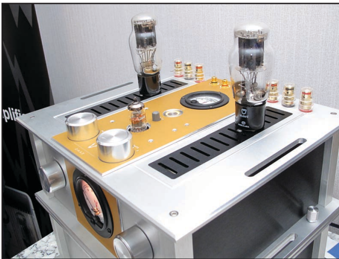
The DAA-3's separate PSU boasts seven low-noise regulated DC supplies.
