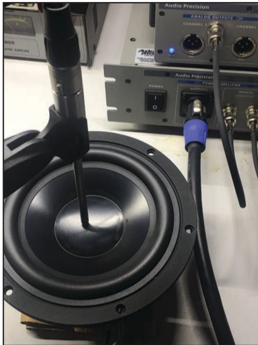
Photo 2: I used the APx515/APx1701 combination to take a nearfield measurement of a 170 mm woofer.
