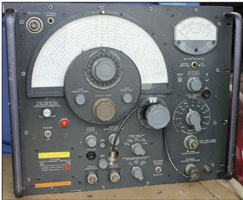
Photo 1: This General Radio sweep-frequency signal generator was only part of a “portable” acoustical test setup in use during the 1960s.
