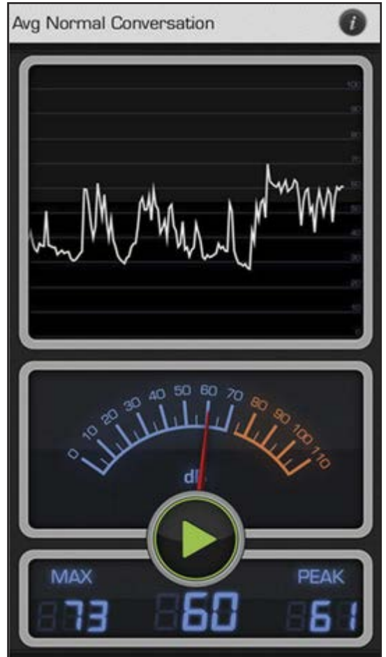
Photo 4: The “Decibel 10th” screen uses a VU-meter-style display.
