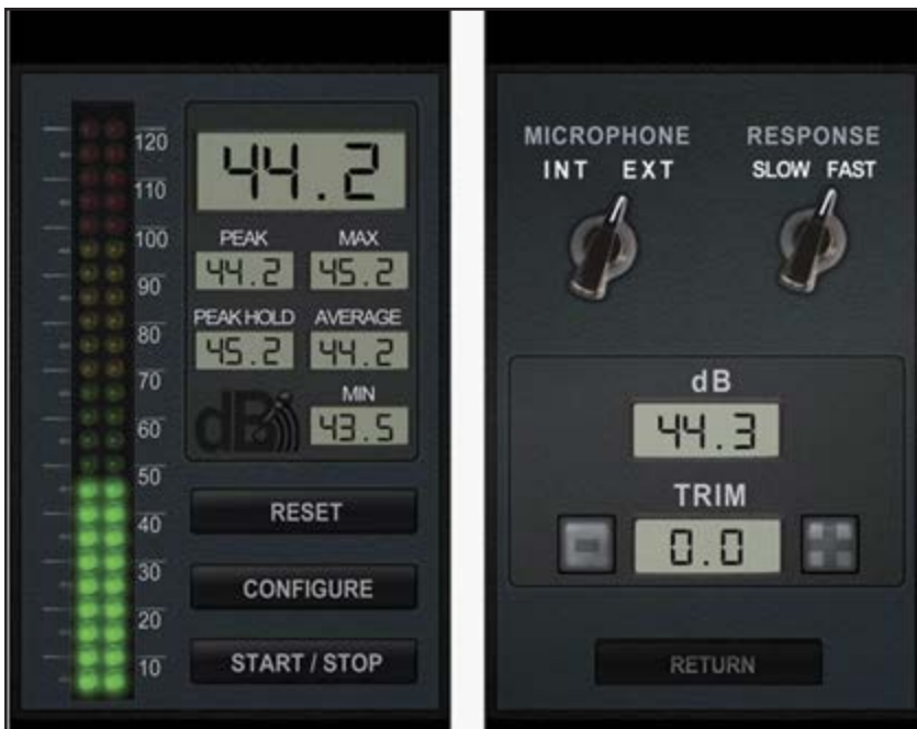
Photo 5: The “dB Volume Meter” shows an LED pictorial-style SPL indication.
