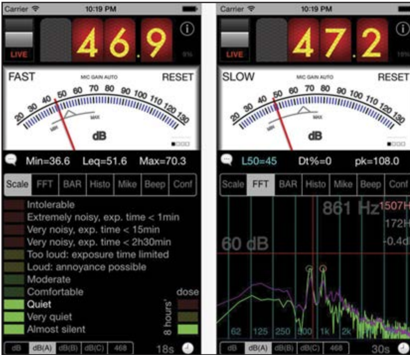
Photo 10: SPLnFFT provides FFT analysis, plus many options for noise measurement.
