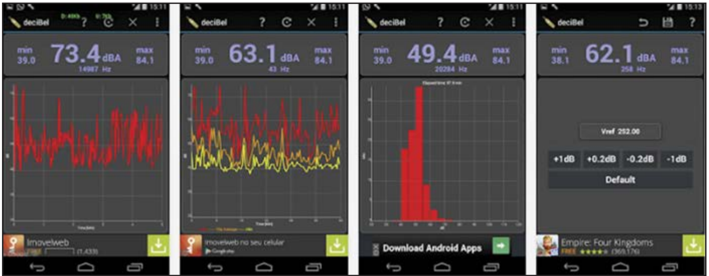
Photo 6: The “decibel” screen can show the values and the waveforms corresponding to the minimum, average, and maximum values of the noise.
