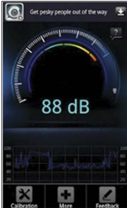
Photo 3: The “Decibel Meter” screen has a speedometer-style sound pressure level (SPL) display.
