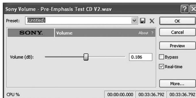
**FIGURE 4:** The FX "Volume" plug-in supplied with Sound Forge allows level adjustments with resolution to 0.001dB.
