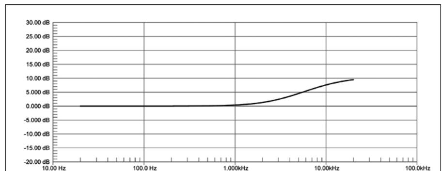
FIGURE 1: The Red Book pre-emphasis curve specifies time constants of 50 $\mu$ S and 15 $\mu$ S. The +3dB point for the high-frequency boost is 3183Hz, shelving at 10610Hz. Maximum boost is +9.49dB at 20kHz.
