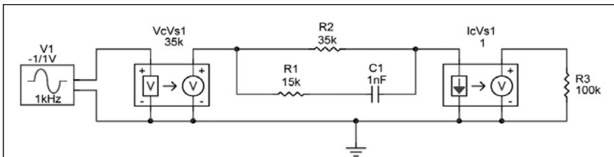
**FIGURE 2:** Simulation model for generating the Red Book pre-emphasis curve. The 50 $\mu$ S time constant is the product of (R1 + R2) \* C1; 15 $\mu$ S is equal to R1 \* C1.
