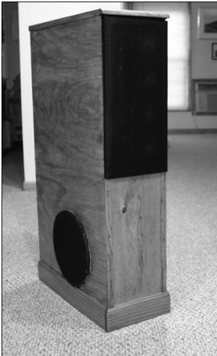
PHOTO 7: Finished enclosure with grille.
