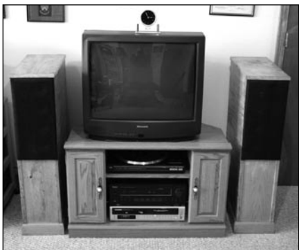
PHOTO 8: Finished enclosure pair.
